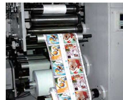
放、收卷均由磁粉自动张力控制 Unwinding and Rewinding Tension are Auto-controlled by Magnetic Powder
