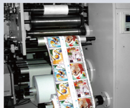
放卷、收卷均自动控制张力 Unwinding and Rewinding Tension are Auto-controlled
